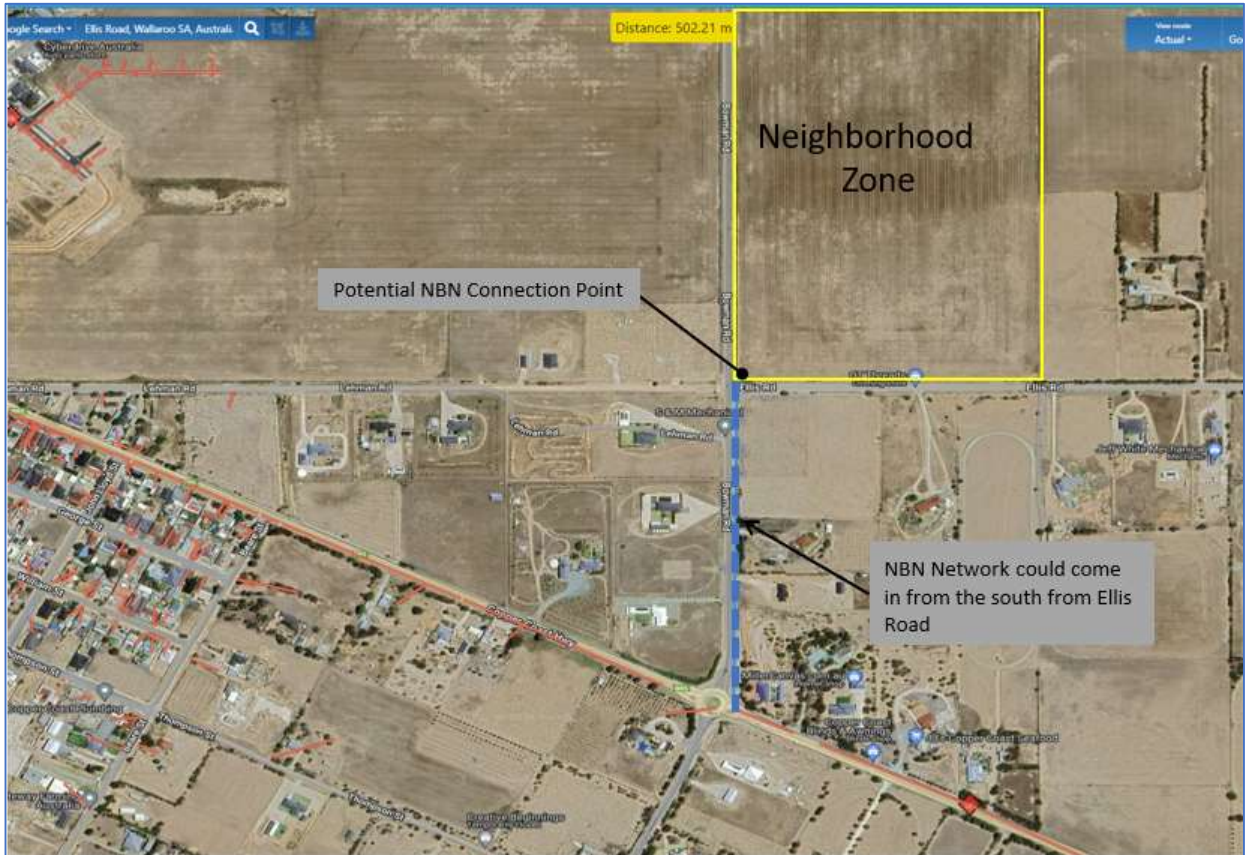
Figure 5: NBN CO possible communications backhaul route
